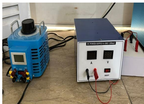
12. High Voltage Power Supply
